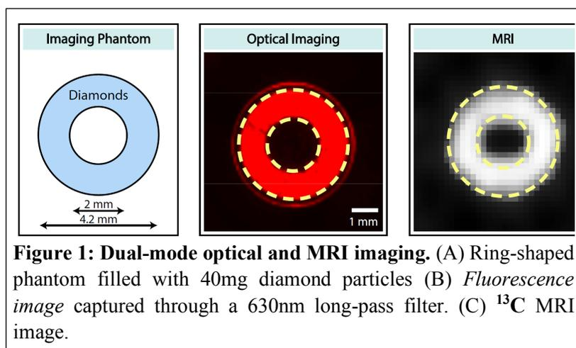
**Figure 1: Dual-mode optical and MRI imaging.** (A) Ring-shaped phantom filled with 40mg diamond particles (B) *Fluorescence image* captured through a 630nm long-pass filter. (C)  $^{13}\text{C}$  MRI image.
